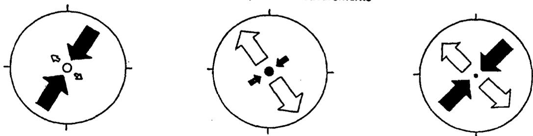
Fig. 9. Mean Quaternary paleostress tensors for the Kurai-Chuya Depression. Symbols displaying horizontal stress axes, with length proportional to their magnitude are as follows. Black inward arrows stand for compressive deviatoric stress and white outward arrows for extensive deviatoric stress. Central symbol is: open circle for compressive regimes, point for strike-slip regimes, black circle for extensive regimes.
