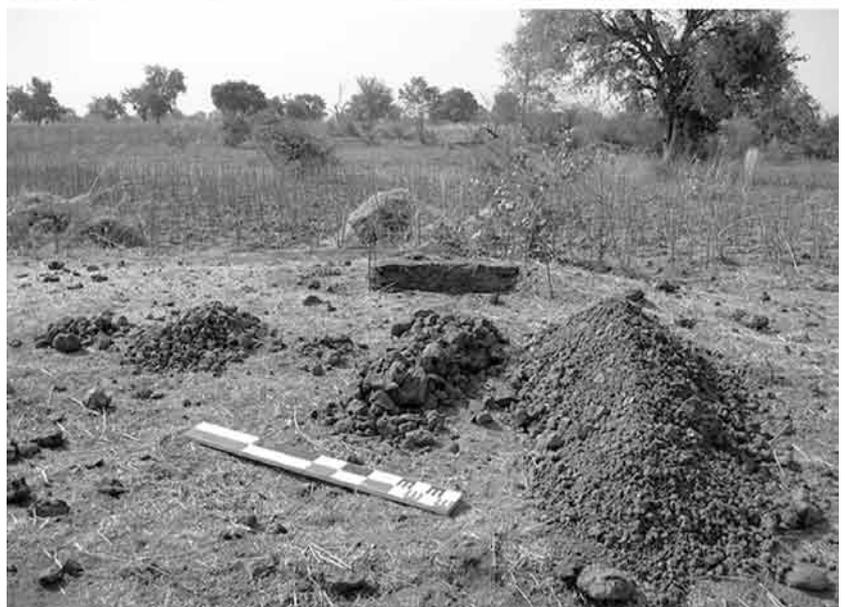
**Fig. 5.** Example of ‘cubing’. All metallurgical waste from a known volume are sorted by category and weighed with a balance. (Photos © Robion-Brunner & Serneels.)
