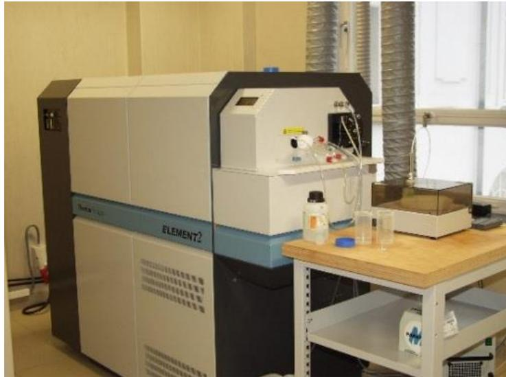
This instrument is a double focusing magnetic sector field ICP-MS with the main following characteristics:
