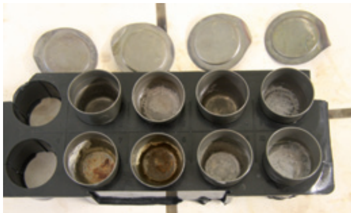
Left: Purification of samples in a 600°C oven. C. Delvaux © RMCA
