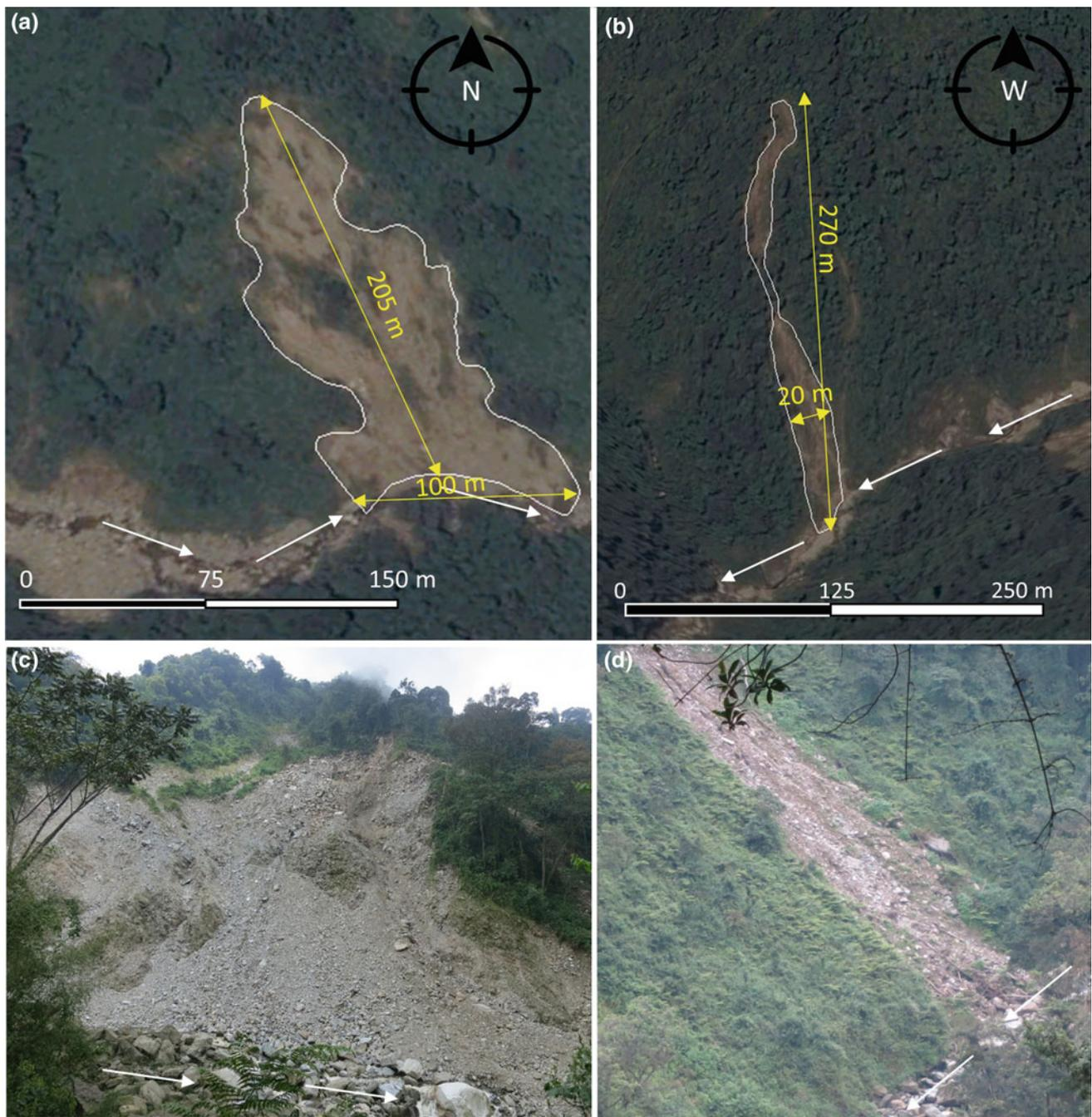
**Fig. 5** Illustration of the two landslide types. **a, c** landslides adjacent to the river with large width-to-length ratios. **b, d** debris flows with a narrow run-out zone. *Top* landslides observed with GE images and
