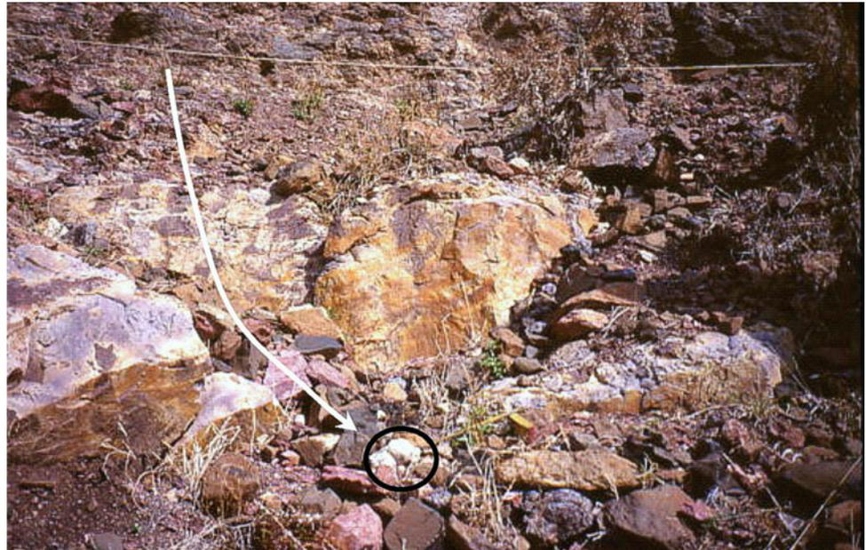
**Table 9.3** Tracer displacement in 20 months, perpendicular to the contour (after Nyssen et al. 2006)
