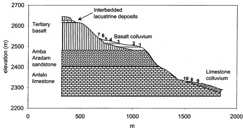
Fig. 4. Geology and location of soil profile pits (1–10).
