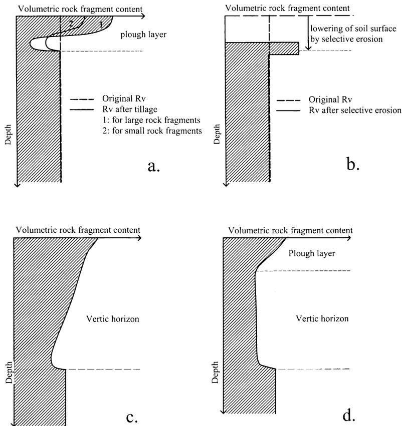
Fig. 2. Theoretical vertical rock fragment distribution as expected to be induced by different processes acting in a soil with an initial homogenous rock fragment distribution: (a) kinetic sieving due to tillage; (b) selective water erosion leading to the development of an erosion pavement; (c) in Vertisols, in chimneys, for larger rock fragments; (d) in Vertisols, in between cracks.
