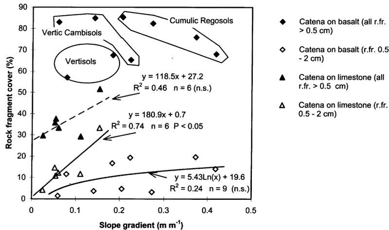
Fig. 8. Slope gradient vs. rock fragment cover, by lithology (average based on six measurements per site). Correlations are improved if only rock fragments <2 cm are taken into account.
