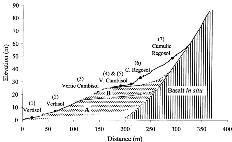
Fig. 10. Soil catena on basalt trapp. Note that most soils are covered by 20–100 cm of recent colluvium (Regosol). Topography was measured by theodolite. See Table 1 for a synthesis of the processes which explain the rock fragment distribution. (A) and (B) are ancient debris flow deposits.
