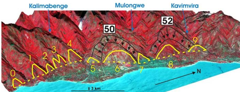
**Fig. 3** 3-D panoramic view of Uvira and part of the mountain hinterland. Fault facets 0–9 in yellow. The head scars of the ancient mega-landslides 50 and 52 in black. Both landslides have been undercut as a result of the downthrow along fault facets 5–9. IKONOS (bands 4, 3, 2 as RGB) draped on the 30 m SRTM, shown in ENVI, Vertical exaggeration:  $\times 2$
