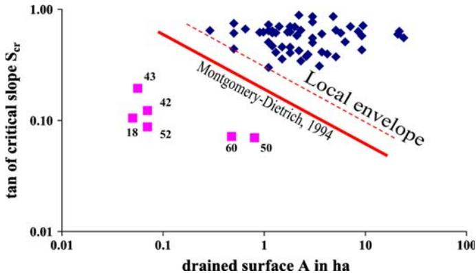
**Fig. 7** The M–D topographic threshold for hillside incisions, as established for America, separates the two groups of landslides at Uvira. If the ‘American’ envelope is shifted to the edge of the right data cloud, it corresponds to the local envelope, established for Rwanda (Moeyersons 2003) where  $S_{cr} \approx 0.3 A^{-0.6}$
