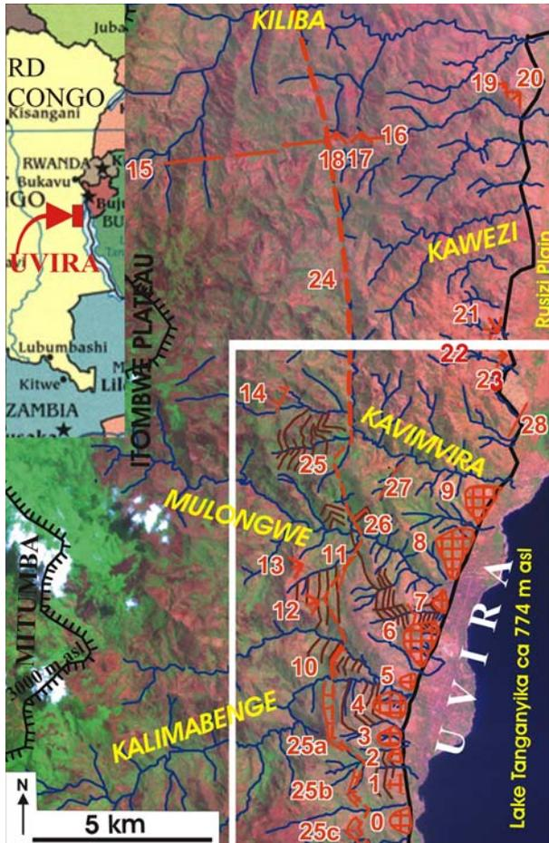
**Fig. 2** The study area. The ETM basic layer is a false colour combination of bands 7, 4 and 2. Band 4 is represented in green so that vegetation is green on the image. Active tectonic structures (Sect. 3.1; Table 1) in red. Blue lines active river incisions (Sect. 3.2). River names in yellow italics. Geologic layers in brown. The heavy black line separates the flat alluvial fans and the Rusizi Plain from the rugged mountains. White frame IKONOS coverage
