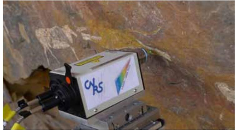
**Fig. 4.** Portable Raman Spectroscopy being used to identify pigments at a rock painting site. Location: Maloti-Drakensberg World Heritage Site, South Africa. (Photo © L. Ronat.)
